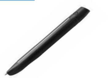
When a G-Pen BT is used for writing on a booklet or a sticker printed with a dot code, the pen strokes are reproduced on a PC or a tablet. Thus, letters and diagrams written on a dedicated dot code sheet can be saved as digital data easily. Furthermore, because of the Bluetooth, there is no need to worry about a USB cable.
